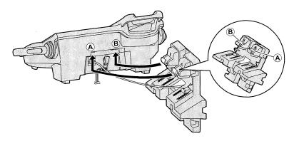
**4** Adjust the adaptor to hold the base unit, then push it in the direction of the arrow until it clicks into place.
